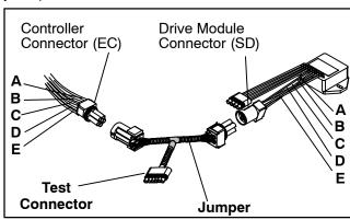
Figure 6-24 Jumper Assembly
