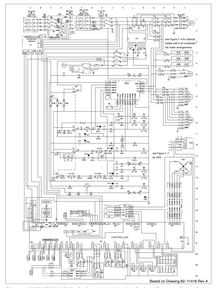
Figure 7-6 SCHEMATIC DIAGRAM - Configuration Includes eAutoFresh and Emergency Bypass Options
