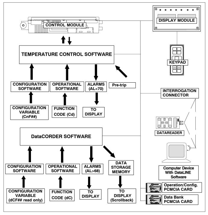
Figure 3-1 Temperature Control System
