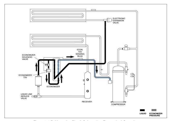
Figure 2-8 Refrigeration Circuit Schematic - Economized Operation
