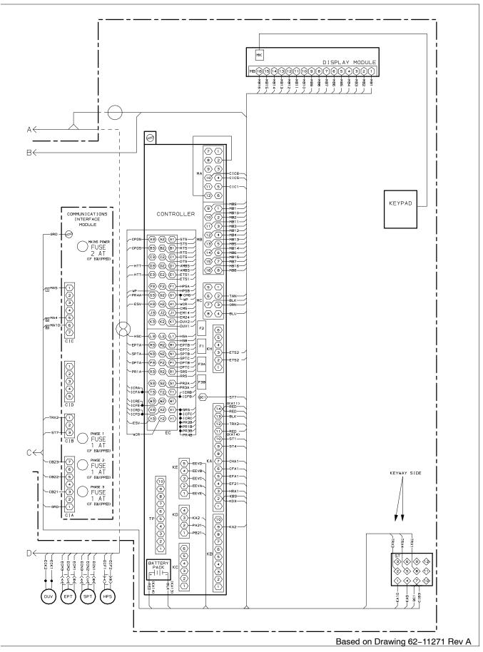
Figure 7–9 UNIT WIRING DIAGRAM – Standard Unit Configuration with 3–Phase Condenser Fan Motors (Sheet 2 of 2)
