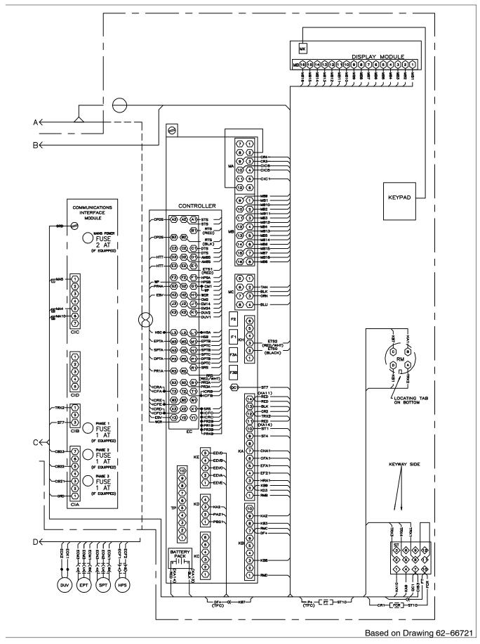
Figure 7-10 UNIT WIRING DIAGRAM - Configuration Includes Single Phase Condenser Fan Motor and Optional Heater Arrangement (Sheet 2 of 2)
