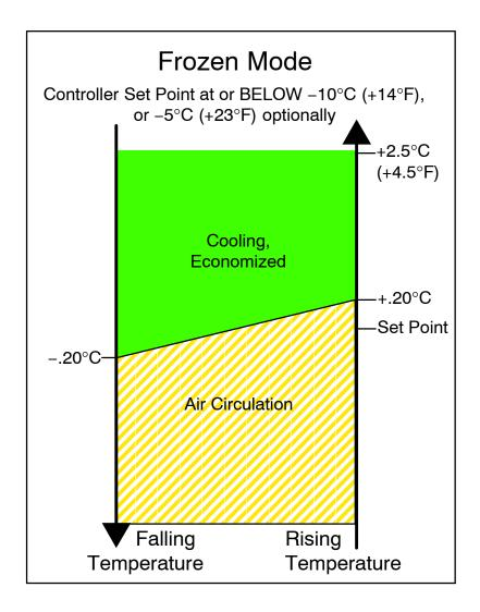
Figure 3-8 Controller Operation - Frozen Mode
