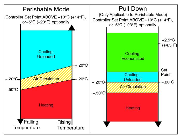
Figure 3-5 Controller Operation - Perishable Mode
