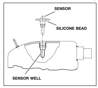
Figure 6–22 Compressor Discharge Temperature Sensor
