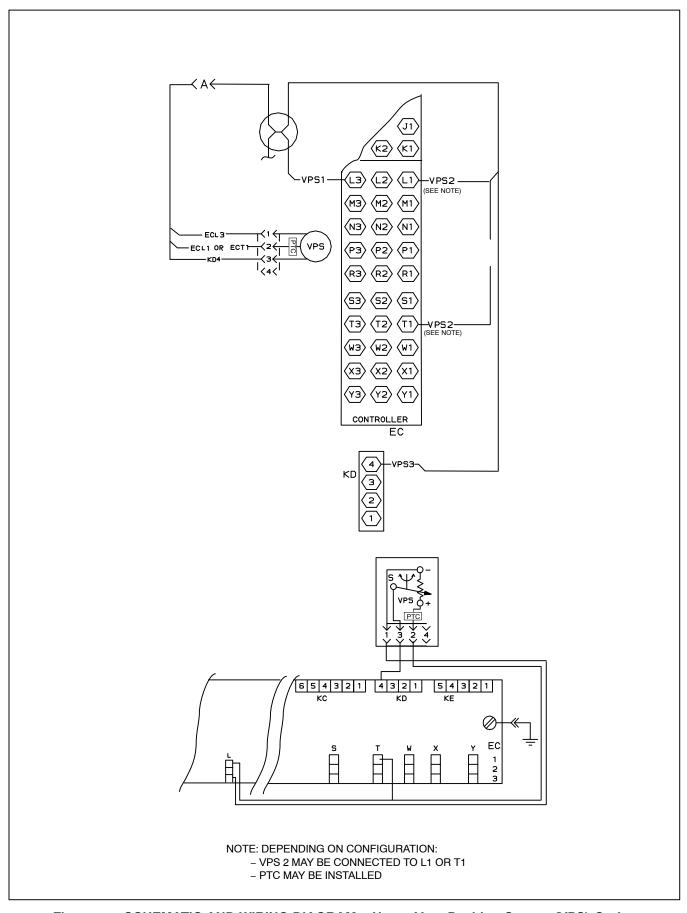
Figure 7-7 SCHEMATIC AND WIRING DIAGRAM - Upper Vent Position Sensor (VPS) Option
