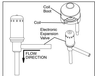
Figure 6-11 Electronic Expansion Valve
