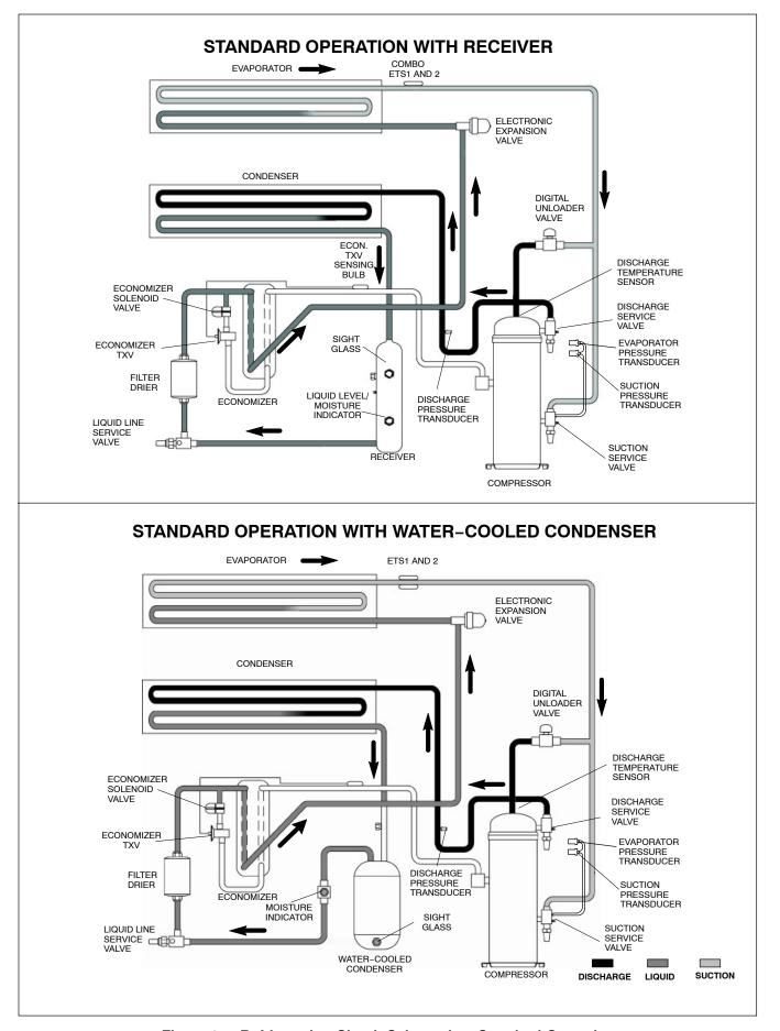
Figure 2-7 Refrigeration Circuit Schematic - Standard Operation
