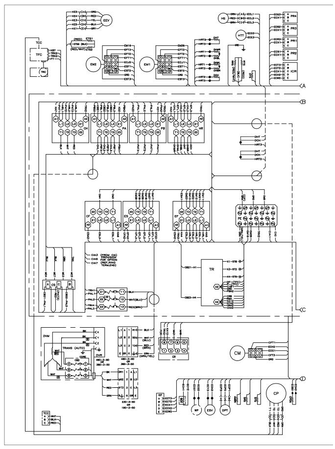
Figure 7-10 UNIT WIRING DIAGRAM - Configuration Includes Single Phase Condenser Fan Motor and Optional Heater Arrangement (Sheet 1 of 2)
