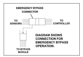
Figure 4–3 Diagram of Emergency Bypass Connections
